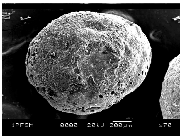
Fig. 2. Scanning electron microphotograph of the optimized calcium pectinate-FSM beads containing metformin HCl prepared through ionotropic gelation (F-O).
